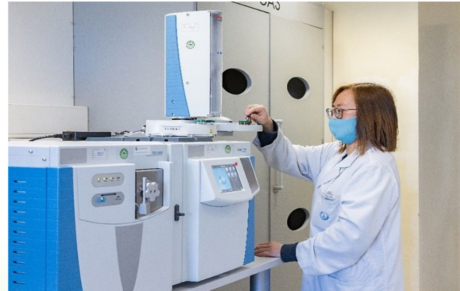
Analyses of organochlorine pesticide residues in pCm samples using gas chromatography-tandem mass spectrometry.
