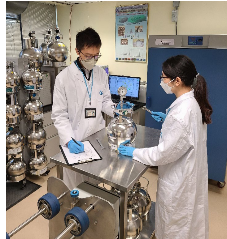
Examination of sample canister prior to the analyses of VOCs in ambient air.
