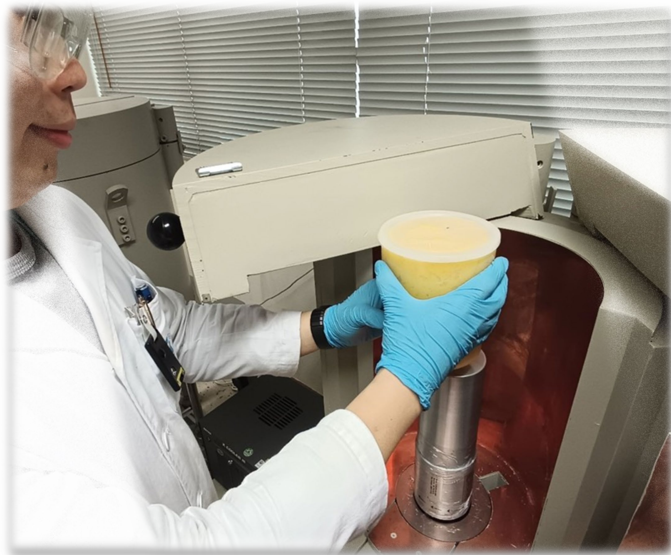
Utilizing gamma-ray spectrometer with high-purity Germanium detector to analyse radionuclide contamination in the imported food samples.
