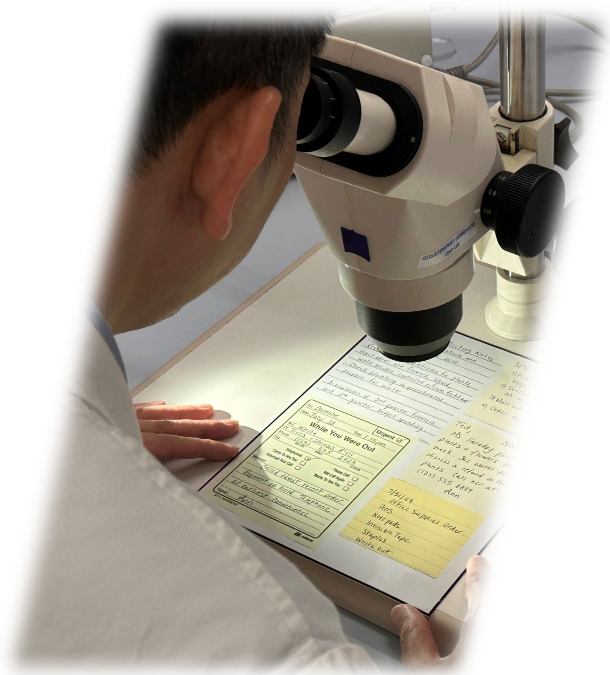
Handwriting examination by stereomicroscopy
