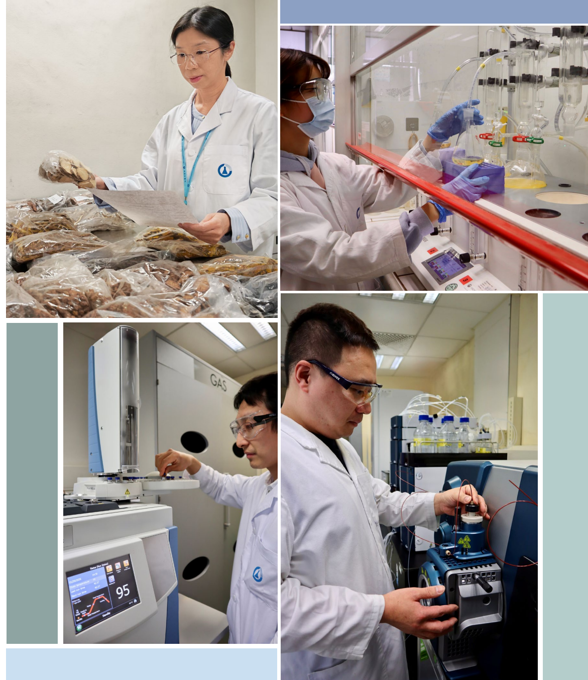
(clockwise from top right) Extraction of sulphur dioxide residue from Chms samples for analysis; Analysis of Chms samples by liquid chromatography-tandem mass spectrometry; Analysis of pesticide residues in Chms samples using gas chromatograph-tandem mass spectrometry; and Verification of Chms samples information.
