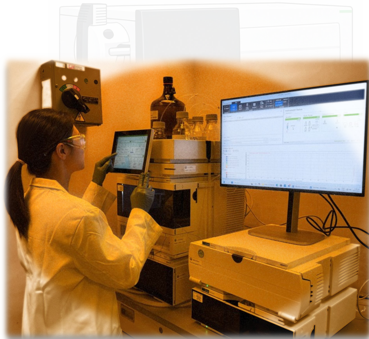
Analysis of active ingredients in vitamin samples by High Performance Liquid Chromatograph system in the vitamin testing laboratory.
