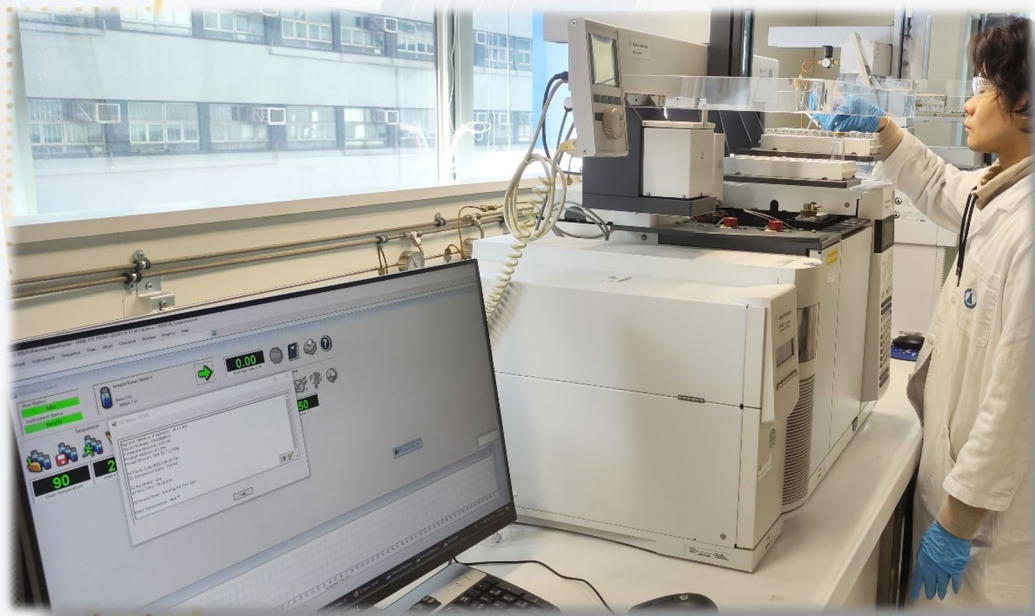
Analysis of preservatives in food samples by gas chromatography-tandem mass spectrometry.
